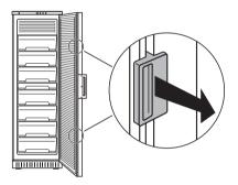
With open door remove transport safeguard at door pivot.
